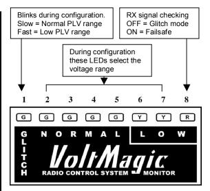
\* There is a 0.1 volt difference between each LED. Using Range 0 for example, LED8 is 4.60 volts or less, LED7 is 4.70 volts, and yellow LED6 is 4.80 volts. A proprietary algorithm accurately dampens changes.
